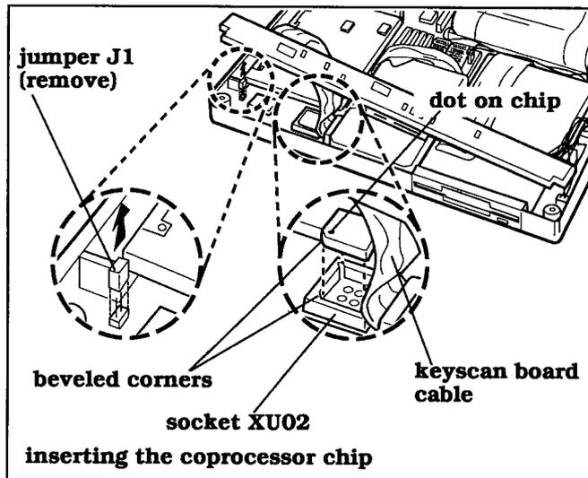
9. Lift up the folded keyscan board cable about 1 inch (25 mm)-but do not disconnect the cable-to gain access to the coprocessor socket (XU02).
