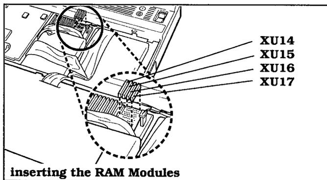
3. Repeat steps 1 and 2 for the remaining three modules in the set, except insert the second module into socket XU15, the third module into socket XU16, and the fourth module into socket XU17.
