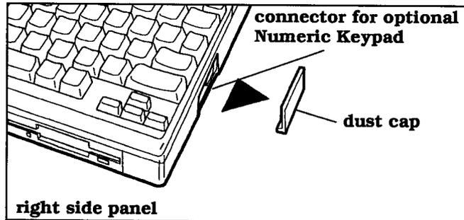
A dust cap is provided for the numeric keypad connector. Remove and store this cap in a safe place while the connector is in use.
