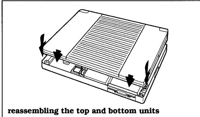
2. Check all around the case to be sure no wires protrude, then press down on the front of the top unit so that it engages with the bottom unit.
