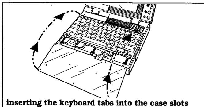
2. Hold the front of the keyboard in place while you lower the rear of the keyboard onto the computer case.
