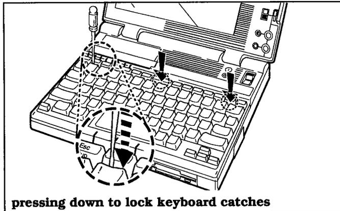
4. Insert the screwdriver blade between the **F8** key and the **7** key and gently press down on the keyboard until the center catch snaps locked.
