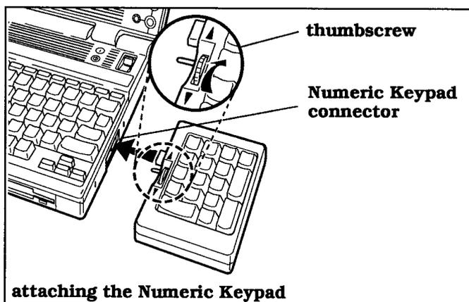
4. Rotate the thumbscrew on the Numeric Keypad clockwise until just tight; do not force.
