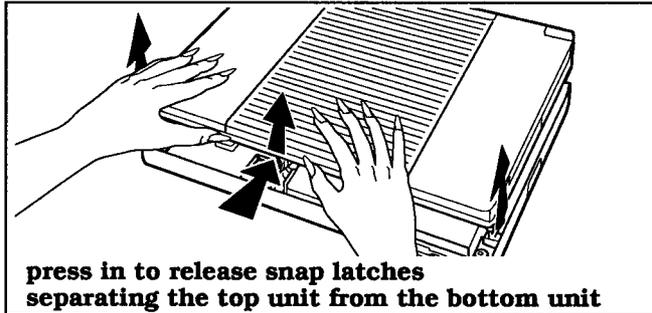
7. Raise the front of the top unit about 2 to 3 inches (50 to 75 mm) to gain access to the coprocessor socket. **Do not separate the rear of the top and bottom units.** The key scan board will likely fall out of the inside front of the top unit.
