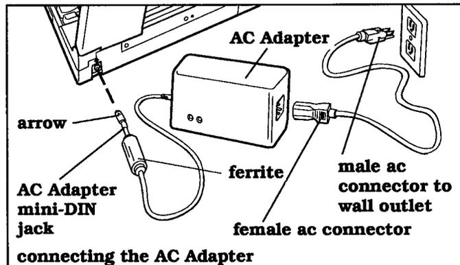
3. Connect the male end of the ac cord into a grounded wall receptacle of the correct voltage. Use a grounded plug adapter if necessary.
