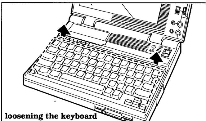
6. Raise the rear of the keyboard several inches, rotate the rear of the keyboard 180 degrees toward you, and place the keyboard in front of you with the keys facing down as shown in the following figure.
